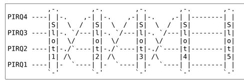
Every PCI card emits a PCI IRQ, which can be INTA, INTB, INTC or INTD:
