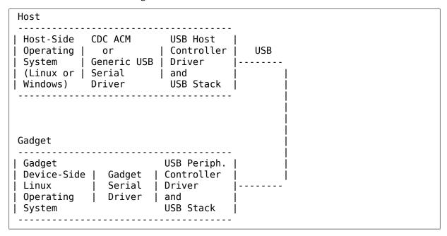
On the device-side Linux system, the gadget serial driver looks like a serial device.
