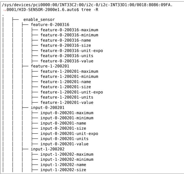
Here there is a custom sensors with four fields, two feature and two inputs. Each field is represented by a set of attributes. All fields except the "value" are read only. The value field is a RW field.
