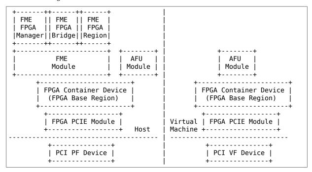
FPGA PCIe device driver is always loaded first once a FPGA PCIe PF or VF device is detected. It:
