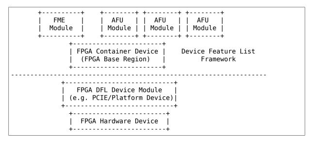
DFL framework in kernel provides common interfaces to create container device (FPGA base region), discover feature devices and their private features from the given Device Feature Lists and create platform devices for feature devices (e.g. FME, Port and AFU) with related resources under the container device. It also abstracts operations for the private features and exposes common ops to feature device drivers.
