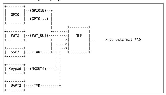
NOTE: the external pad is named as MFP\_PIN\_GPIO19, it doesn't necessarily mean it's dedicated for GPIO19, only as a hint that internally this pin can be routed from GPIO19 of the GPIO controller.
